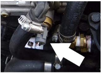
Remove the retainer clip for the LPG fuel temperature sensor and remove the sensor from the regulator body.
