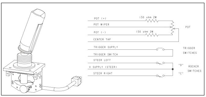
Figure 3-43. Joystick Controller - (JLG P/N 1600308)
