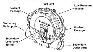
Figure 3-39. Pressure Regulator Section
