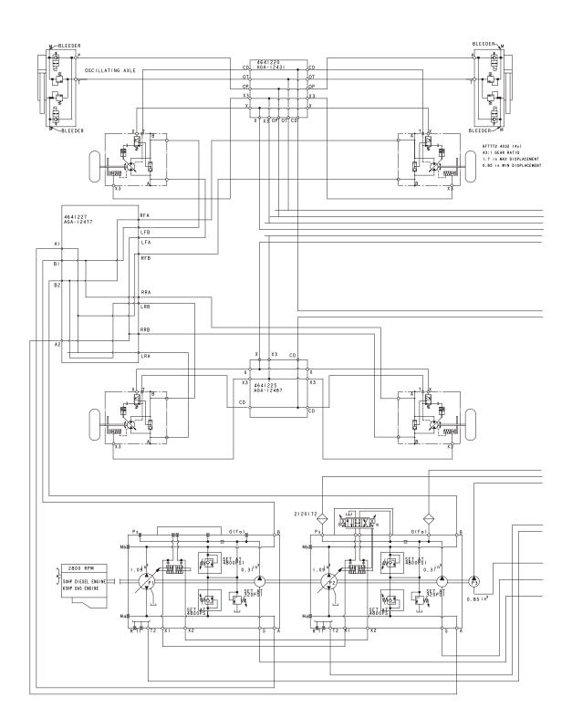
Figure 6-32. Hydraulic Schematic 4WD - Sheet 1 of 4
