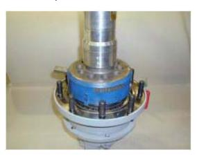
11. After proper bearing setting is completed, hammer ball with suitable punch, 1.1 - 1.3mm into the spindle thread. Retain ball in position with expanding plug.
