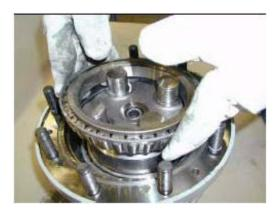
De-grease threads of Spindle (34) and Shaft Nut (4).
