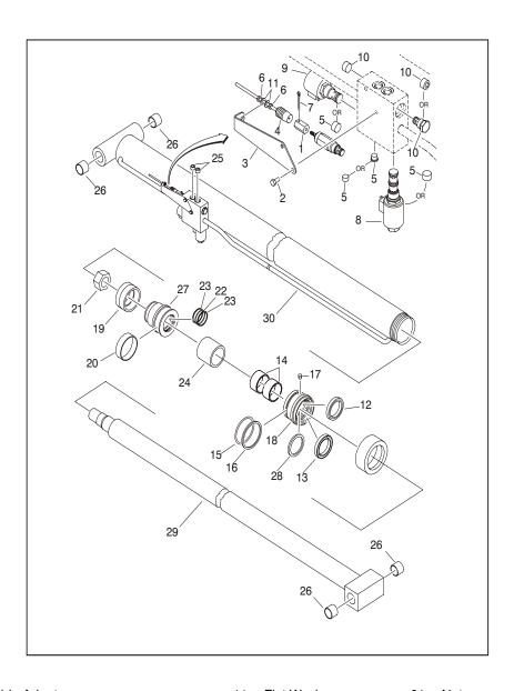
1. Cable Adapter 11. Flat Washer 21. Nut Bolt Wiper Seal 2. 12. 22. 3. Bracket 13. Seal 23. Ring, Back-Up Manual Descent Cable Ring, Wear Spacer 14. 24. 5. Plug, O-Ring 15. Seal Plug, O-Ring 25. 6. Jam Nut 16. Ring, Back-Up Bushing 26. 7. Cotter Pin 17. Setscrew 27. Piston 8. Cartridge, Lift Holding Solenoid 18. Head 28. Seal 9. Cartridge, Lift Holding Solenoid 19. Seal 29. Rod 10. Cartridge, Check 30. Barrel 20. Ring, Wear
