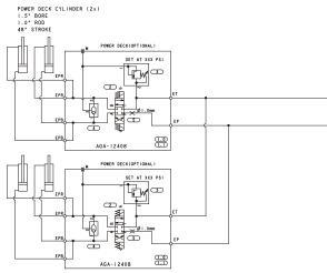
Figure 6-38. Hydraulic Schematic 2WD - Sheet 3 of 4
