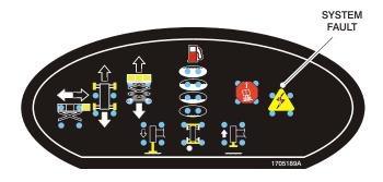
NOTE: Flash codes are also displayed on the handheld analyzer. For descriptions see Table 5-1, Fault Code Listing.
