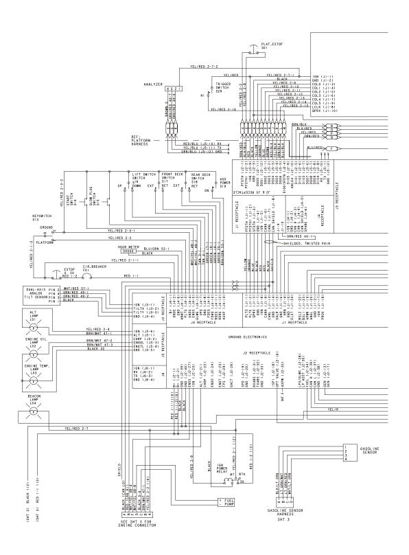
Figure 6-24. Electrical Schematic - Dual Fuel GM - Sheet 1 of 5
