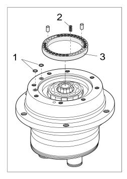
4. Disassemble retaining ring.
