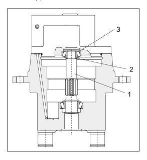
30. Place measuring device. Ascertain tolerance. Grip shaft with Seeger ring pincers and move up and down. [Simulation ring 1mm + tolerance + (bearing pretension 0.05 - 0.08) is resulting in thickness of the synchronizing disc]. Grind synchronizing disc to dimension.
