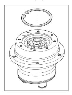
5. Disassemble bearing with synchronizing plate.
