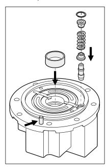
16. Fix control plate with grease at port plate.
