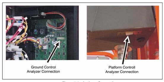
Figure 5-2. Analyzer Connection
