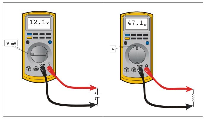
Figure 6-1. Voltage Measurement (DC)
