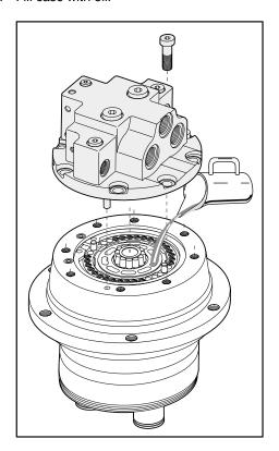
18. Mount and screw port plate on supporting axle.
