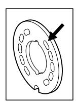
22. Check splines (1) for damage or fretting; running surfaces (2);groove cut by shaft seal (3).
