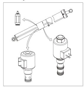
Figure 4-1. Lift Cylinder Holding Valve and Fitting Removal
