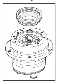
8. Disassemble lamination kit.
