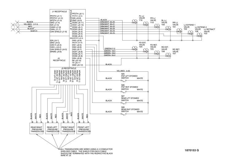
Figure 6-23. Electrical Schematic Diesel (Prior to S/N 138634) - Sheet 3 of 3
