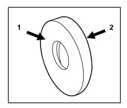
24. Make sure the seat of the shaft seal in the case has no damage.
