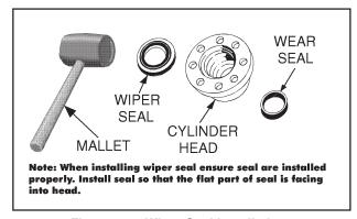
Figure 4-9. Wiper Seal Installation
