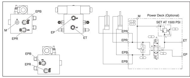
Figure 4-23. Power Deck Manifold Valve
