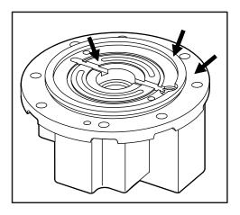
26. Press bearing ring in port plate (with tool).
