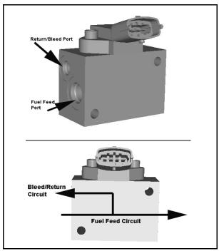
Figure 3-36. Gasoline Fuel Pressure and Temperature Manifold Assembly
