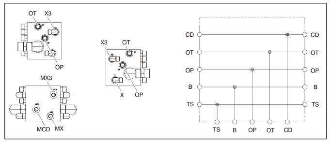
Figure 4-20. Header Valve (Osc)
