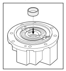
27. Press bearing ring in supporting axle (with tool).
