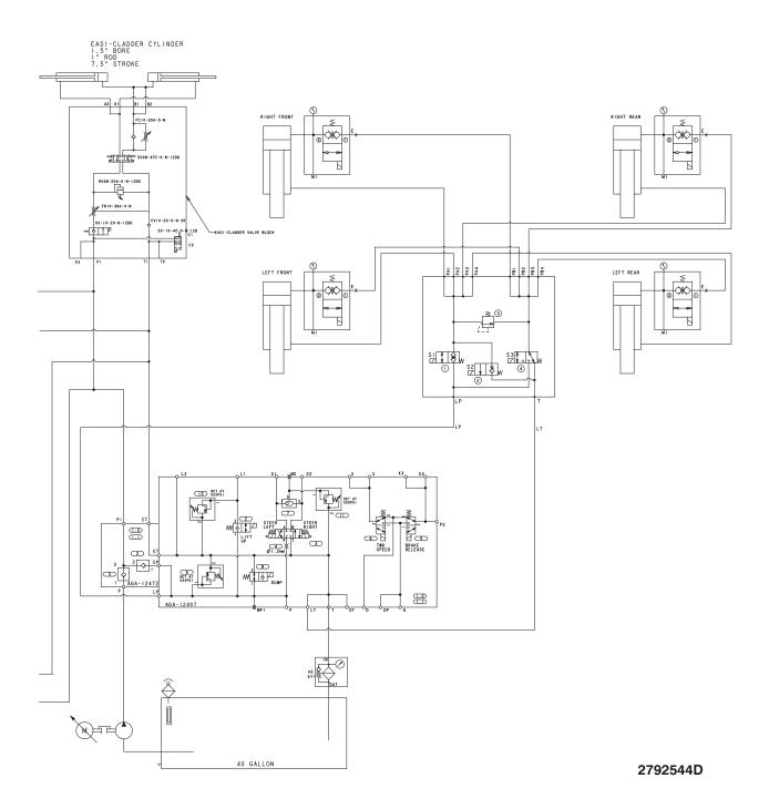
Figure 6-39. Hydraulic Schematic 2WD - Sheet 4 of 4
