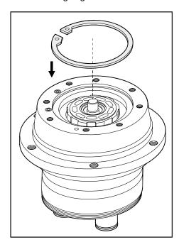
12. Mount seal rings (1). Insert and line-up guide ring.
