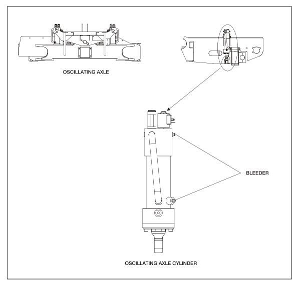
Figure 4-34. Oscillating Axle Bleeding
