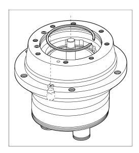
5. Fit pressure pins using an assembly aid. Pre-tension the spring using a suitable device.
