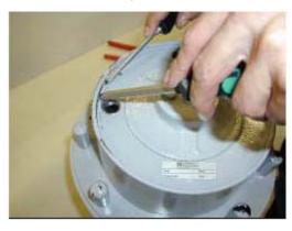
3. Remove the assembled Cover (8) with Shift Rod (33) and O-ring (23).
