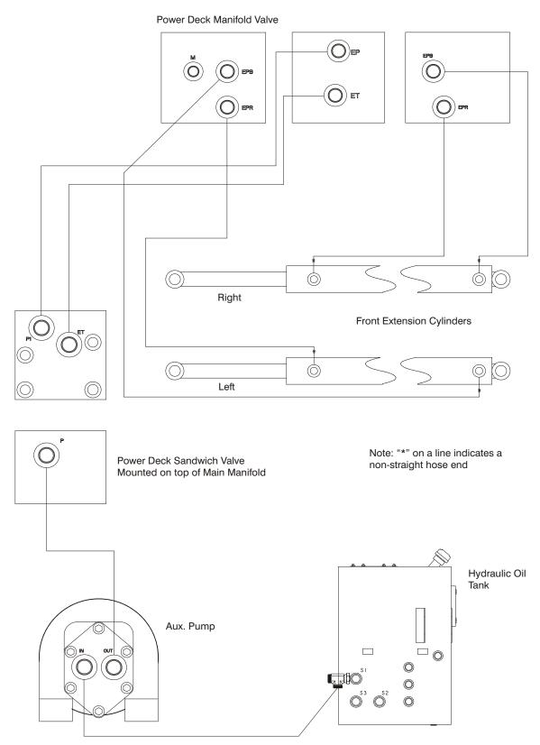
Figure 6-43. Hydraulic Diagram - Deck Extension (Single)
