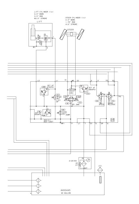
Figure 6-33. Hydraulic Schematic 4WD - Sheet 2 of 4
