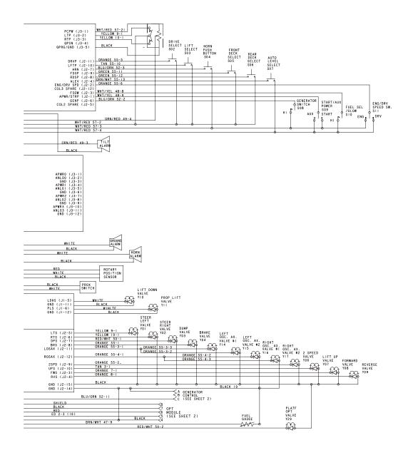
Figure 6-25. Electrical Schematic - Dual Fuel GM - Sheet 2 of 5
