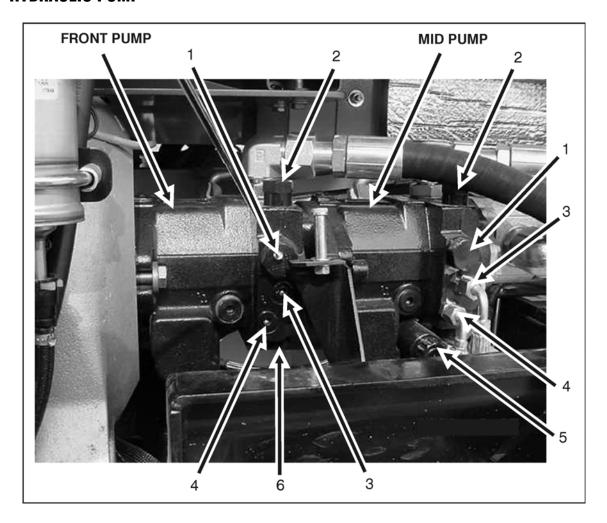
Figure 4-24. Pump Pressure Locations
