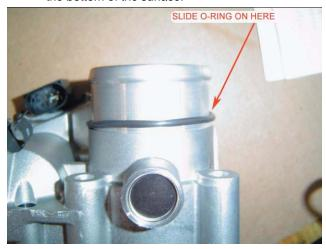
Install the two quad seals. Install one seal at a time to insure the seal does not roll. The seal must sit flat on the throttle body.
