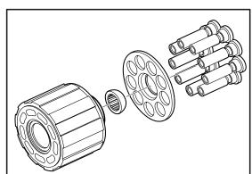
7. Assembly aid: Hold the pistons by using an o-ring.
