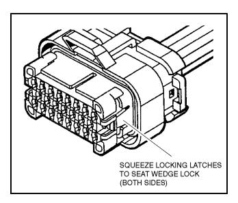
Figure 6-8. Connector Assembly (3 of 4)
