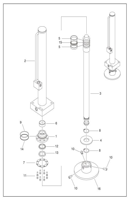
Figure 4-32. Leveling Jack Cylinder
