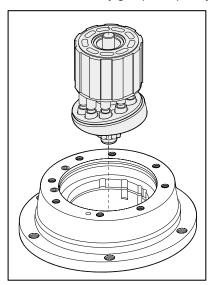
12. Disassemble control piston with spring.
