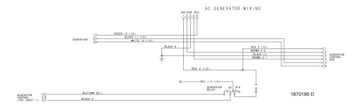
Figure 6-31. Electrical Schematic Diesel (S/N 138634 to Present) - Sheet 3 of 3
