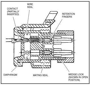
Figure 6-6. Connector Assembly (1 of 4)
