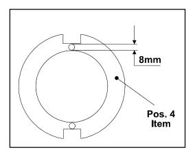
11. Split the Shaft Nut (4) in the area of the two drill holes by means of a chisel, and remove from Spindle (34).
