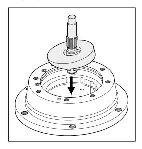
3. Mount sleeve and pressure ring in cradle stop. Insert cradle stop.
