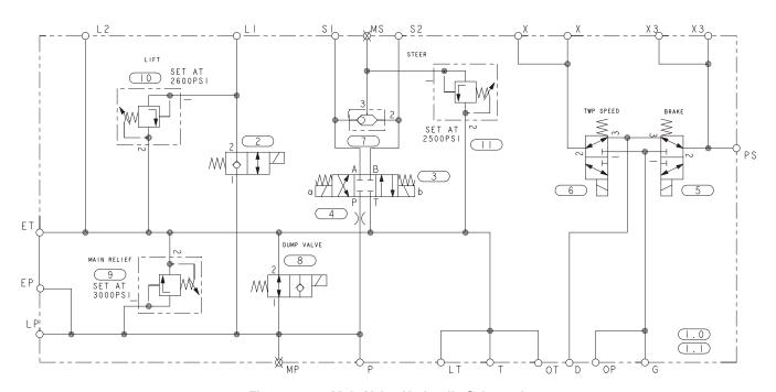
Figure 4-16. Main Valve Hydraulic Schematic
