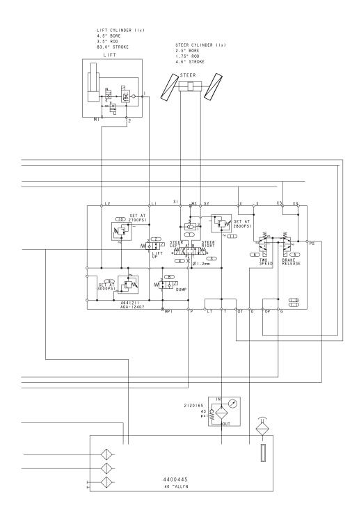
Figure 6-37. Hydraulic Schematic 2WD - Sheet 2 of 4
