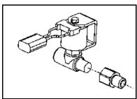
Figure 3-28. Electric Fuel Lock Off
