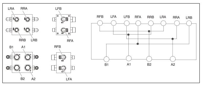
Figure 4-18. Drive Header Valve (4wd)
