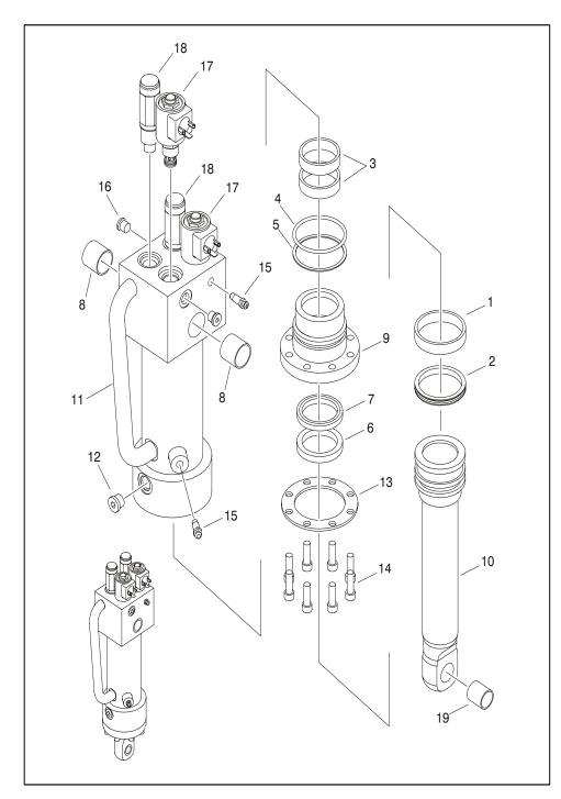
Figure 4-30. Oscillating Axle Cylinder
