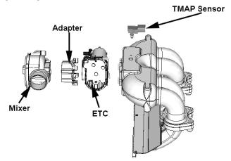
Figure 3-40. (TMAP) Sensor & Electronic Throttle Control (ETC)
