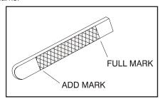
Figure 3-26. Engine Oil Dip Stick
