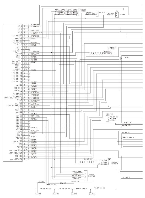
Figure 6-27. Electrical Schematic Dual Fuel - GM - Sheet 4 of 5
