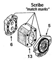
Before beginning disassembly, scribe "match marks" on the body (13) and covers (5 and 6) to insure that the pump will be reassembled in the same manner as it was shipped from the factory. If the body or rear cover is replaced during overhaul, scribe a match mark on the new part in the same location as on the part it replaced.
