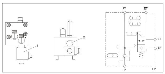
Figure 4-22. Power Deck Sandwich Valve (Dual Deck Extension Only)
