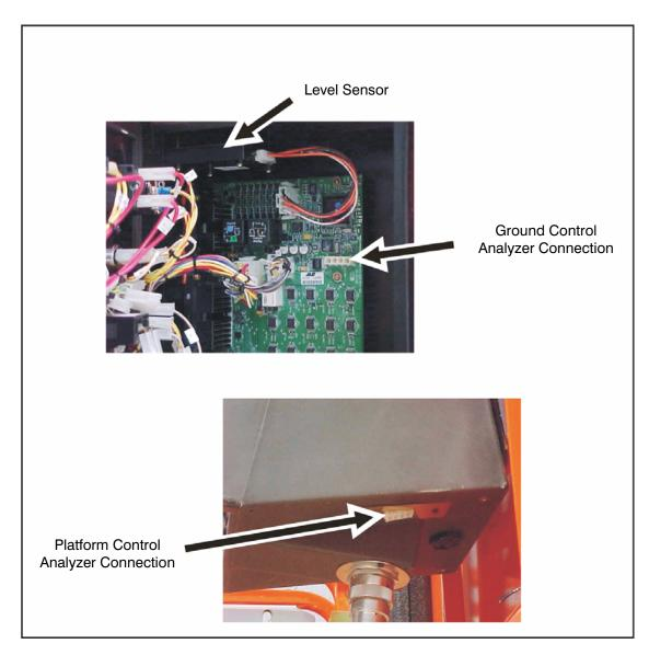
Figure 3-2. Level Sensor and Analyzer Connections
