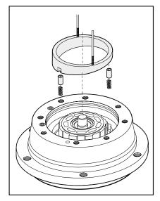
11. Disassemble rotary group completely with cradle.
