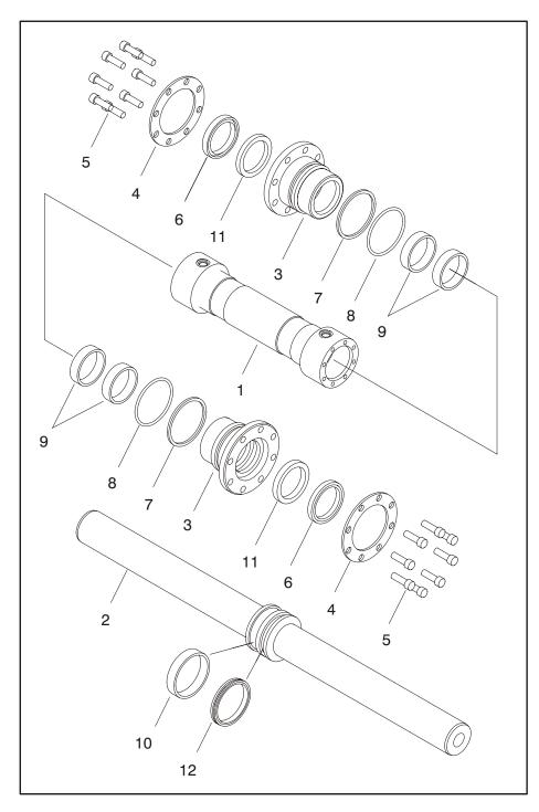
Figure 4-26. Steer Cylinder - Prior to S/N 137518
