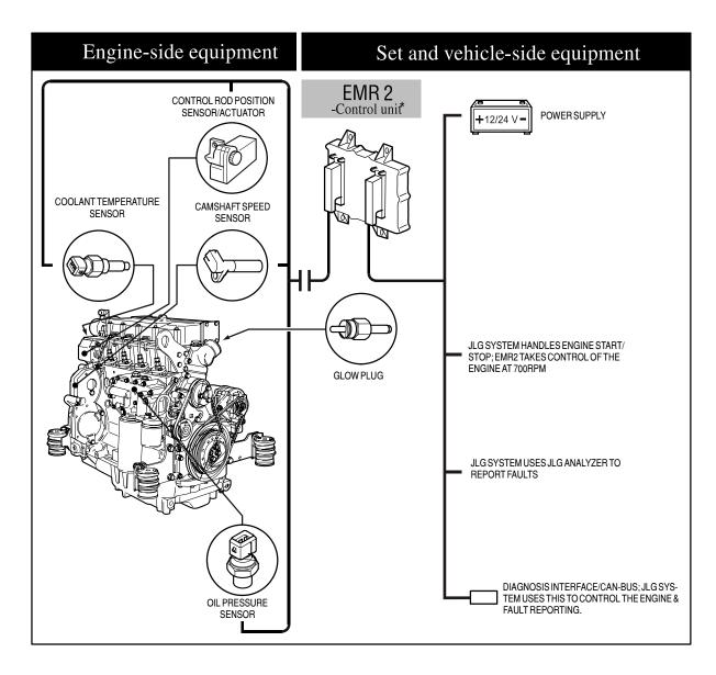
Figure 3-13. EMR 2 Engine Side Equipment
