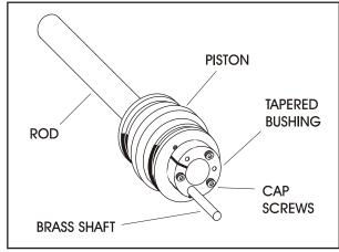
Figure 4-13. Seating the Tapered Bearing
