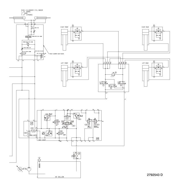
Figure 6-35. Hydraulic Schematic 4WD - Sheet 4 of 4
