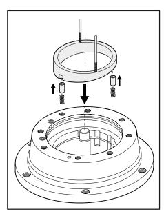
4. Mount Seeger snap ring. Opening of snap ring must be on the opposite side of the control piston.
