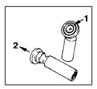
20. Check cylinder bores, splines.
