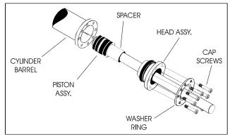
Figure 4-14. Rod Assembly Installation
