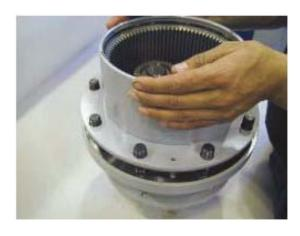
15. Install the ring gear hex head bolts. Tighten bolts to proper torque of 15.5 ft-lbs (21 Nm).
