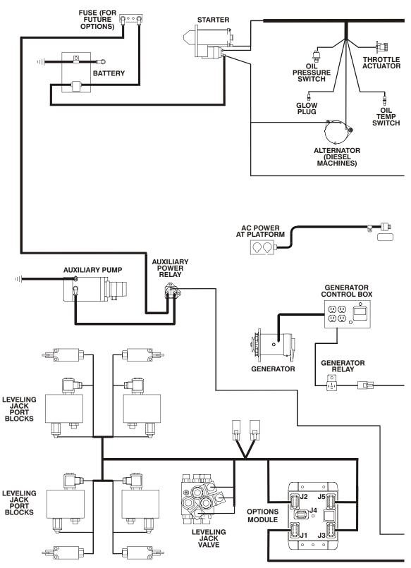
Figure 6-46. Electrical Components Installation - Sheet 1
