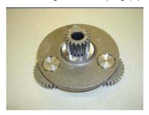
**NOTE:** Heat Supporting Ring (6) up to approximately 189.5°F/70°C in a heating furnace.
