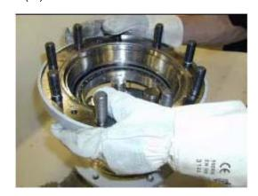
Heat upper ring with roller cage of double Tapered Roller Bearing (11) to approximately 189.5°F/70°C and mount onto Spindle (34). Allow cooling time of approximately 15 minutes before continuing assembly.
