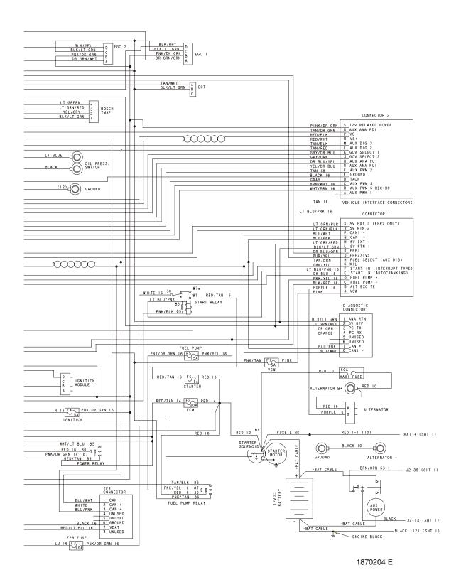
Figure 6-28. Electrical Schematic Dual Fuel - GM - Sheet 5 of 5
