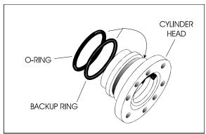
Figure 4-10. Installation of Head Seal Kit
