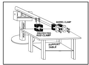
Figure 4-2. Cylinder Barrel Support
