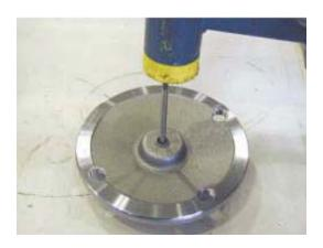
21. Install preassembled Cover (8) into Ring Gear (22).
