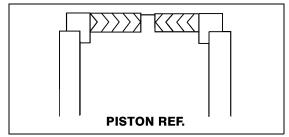
Figure 4-8. Poly-Pak Piston Seal Installation
