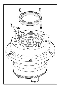
13. Align the two holes for fixation cylinder pin - port plate (item 2).
