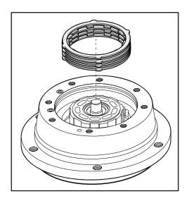
9. Mount support ring (1) and quad ring (2) in pressure ring. Be careful not to excessively extend the rings.
