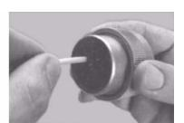
Figure 6-14. HD/HDP Contact Installation
