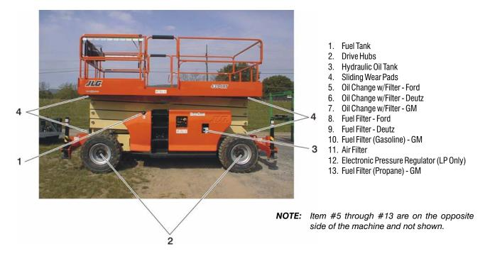
Figure 1-2. Operator Maintenance and Lubrication Diagram
