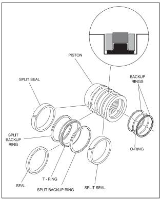
Figure 4-11. Piston Seal Kit Installation
