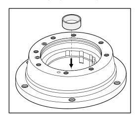
28. Press bearing on drive shaft.
