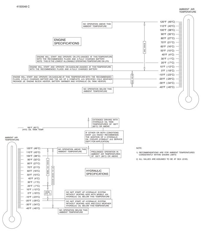
Figure 2-3. Engine Operating Temperature Specifications - GM
