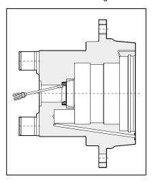
15. Insert disc. Pull off bearing ring with device. Remove disc.
