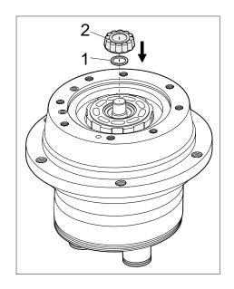
15. Mount bearing ring with device. Mount spool. Mount fixation pin.
