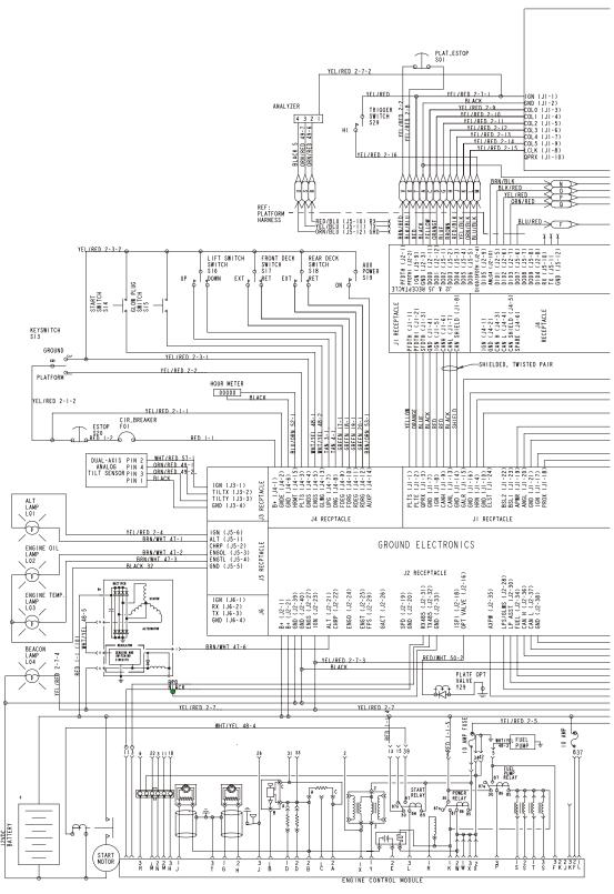
Figure 6-18. Electrical Schematic - Dual Fuel - Sheet 1 of 3
