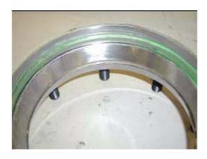
4. Coat bore in Supporting Ring (6) with Loctite 573 for Radial Shaft Seal Ring (17).
