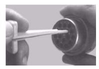
Figure 6-16. HD/HDP Contact Removal
