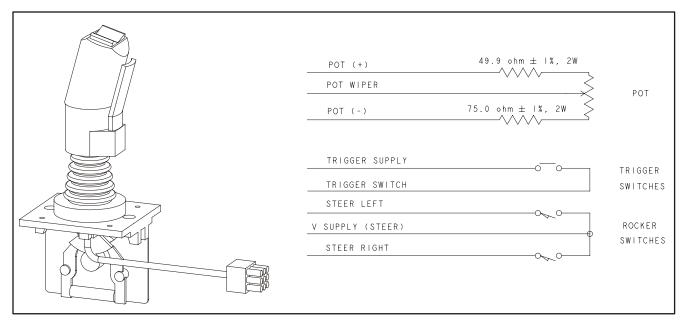
Figure 3-44. Joystick Controller - (JLG P/N 1600403)
