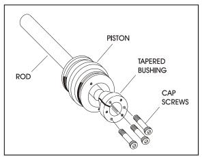
Figure 4-5. Tapered Bushing Removal
