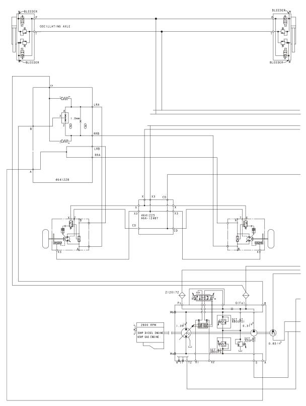
Figure 6-36. Hydraulic Schematic 2WD - Sheet 1 of 4
