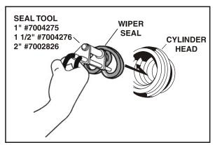
Figure 4-7. Rod Seal Installation
