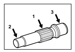
23. Check that sliding surface is free of grooves (1); cups are free of groove and there are no pittings (2).
