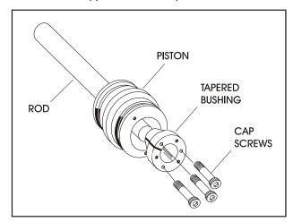
Figure 4-12. Tapered Bushing Installation
