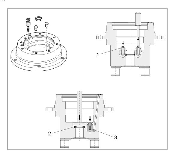
2. Install rotary group with cradle. Observe installation position of swivel balls.
