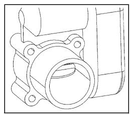
Figure 3-32. ETC throttle control device
