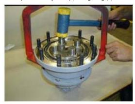
13. Remove Radial Shaft Seal Ring (17).
