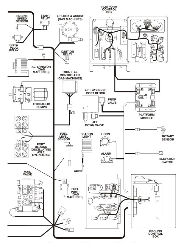
Figure 6-47. Electrical Components Installation - Sheet 2
