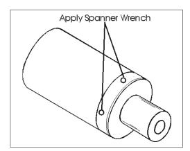
Figure 4-3. Lift Cylinder Cap Screw Removal
