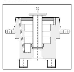
16. Disassemble bearing ring from port plate.
