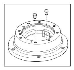
14. Disassemble shaft seal ring.
