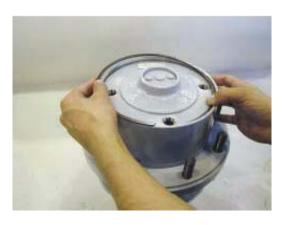
**NOTE:** Prior to putting into operation fill the drive with new oil.
