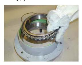
6. Insert radial Shaft Seal Ring (17) into Supporting Ring (6) and fill mounting space between sealing lips with roller bearing grease.
