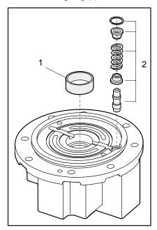
18. Disassemble shuttle valve (1). Disassemble throttle screw with throttle pin (2).
