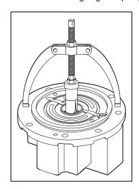
17. Remove bearing ring (1). Disassemble spool (2).
