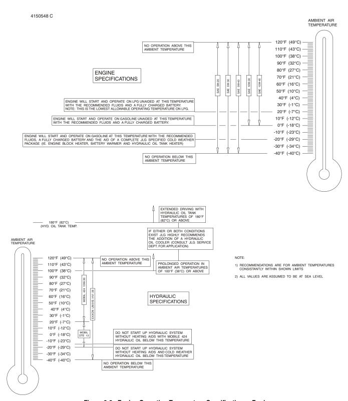
Figure 2-2. Engine Operating Temperature Specifications - Ford
