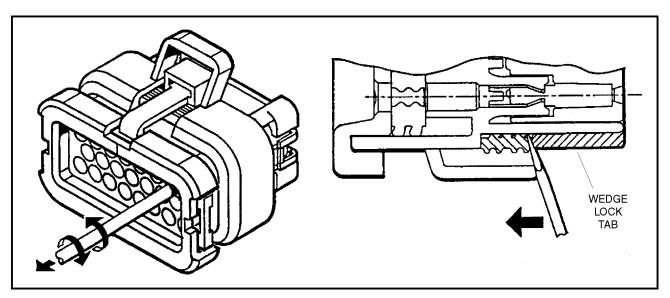
Figure 6-10. Connector Disassembly
