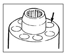
21. Check that cylinder track is free of scratches, there are no traces of wear and no embedded foreign particles. Make sure there are no scratches on the valve plate. (Replace ONLY in sets).
