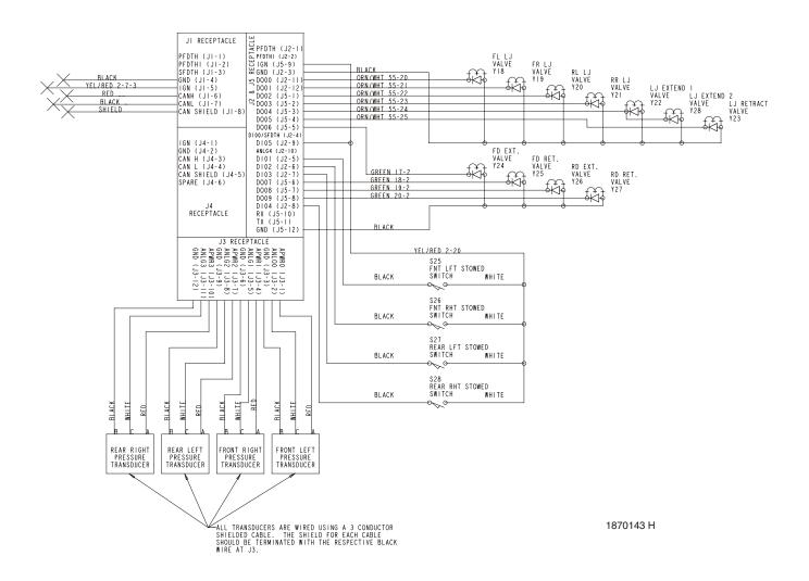
Figure 6-20. Electrical Schematic - Dual Fuel - Sheet 3 of 3
