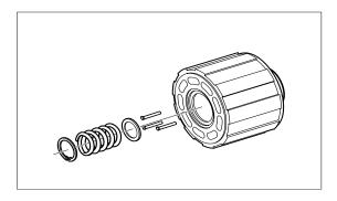
6. Assemble piston with retaining plate. Oil piston and slipper pad.
