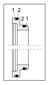
10. Grease seal rings, install in supporting axle.
